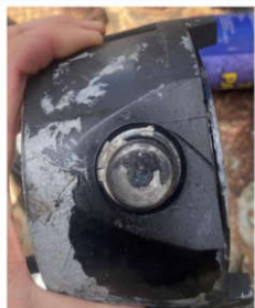
Figure 2. Plugged pressure gauge from the incident.
